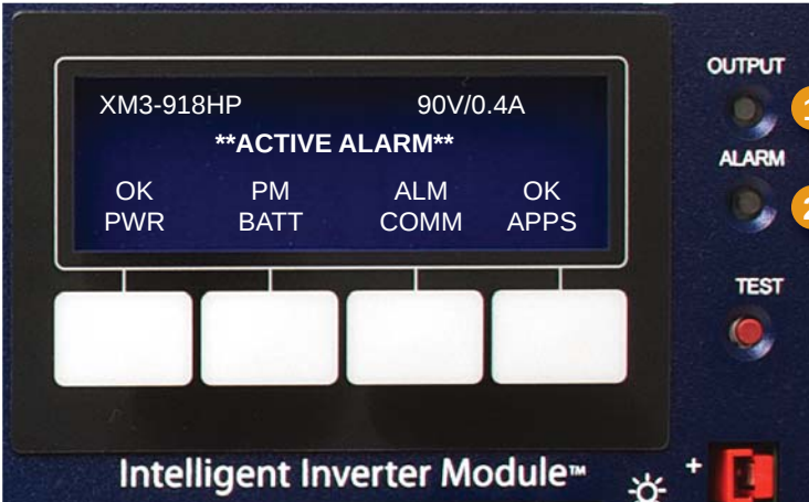
1 OUTPUT LED (green) 2 ALARM LED (red)
