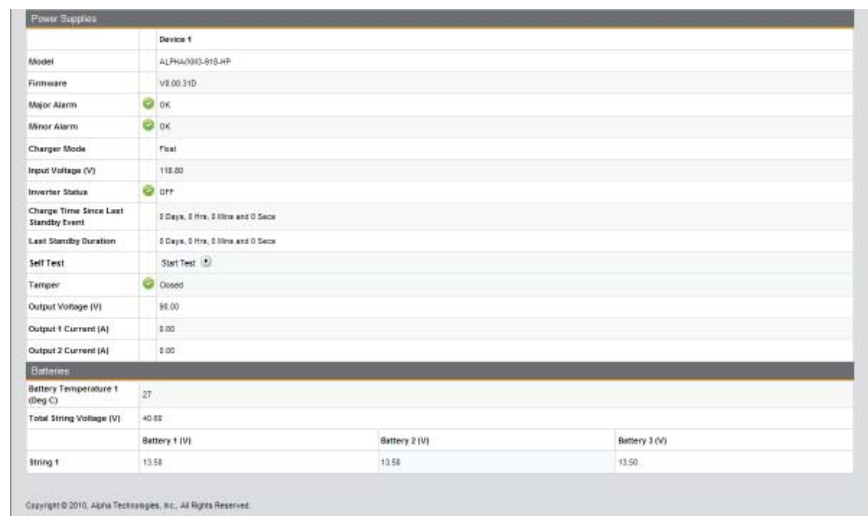
Fig. 2-20, Power Supply and Battery Parameters (data values shown for illustration purposes only)
