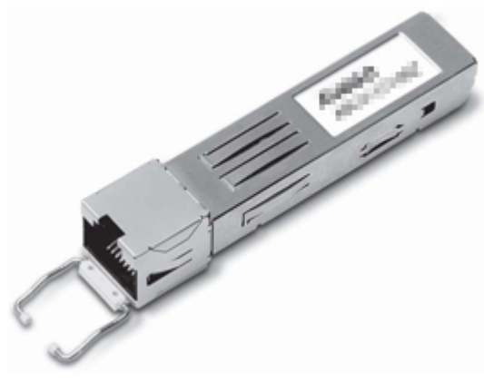
Figure 1-96 1 Gbit/s electrical transceiver
