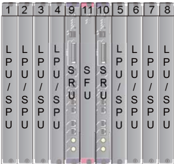
Figure 1-21 AntiDDoS8080 slot layout
