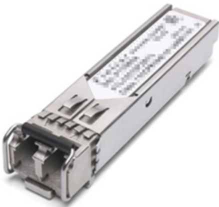
Figure 1-99 10 Gbit/s SFP+ optical module
