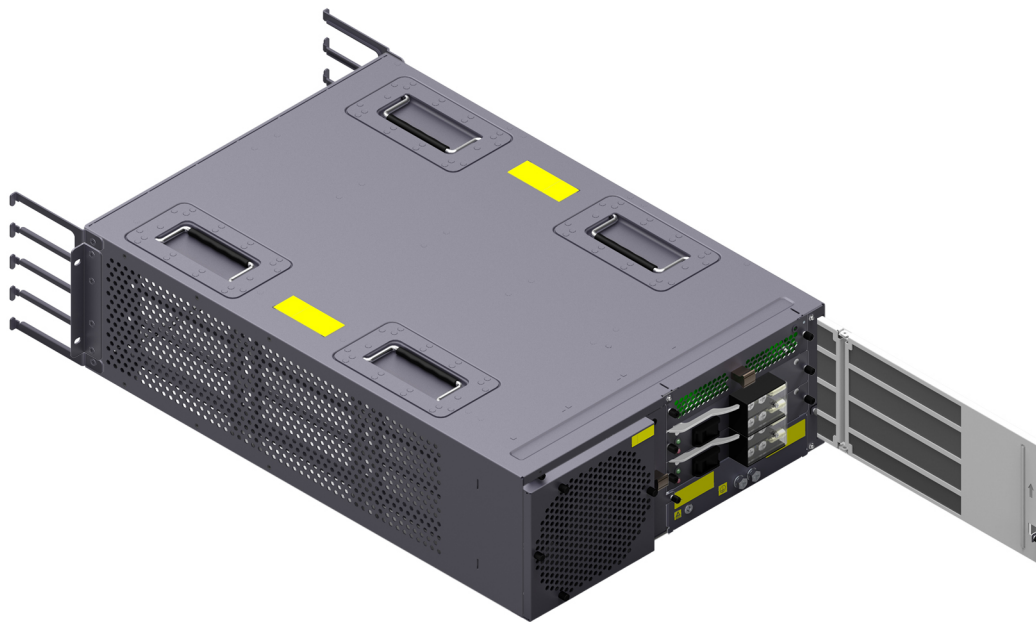
Figure 1-46 Air filter on the AntiDDoS8030 air intake frame
