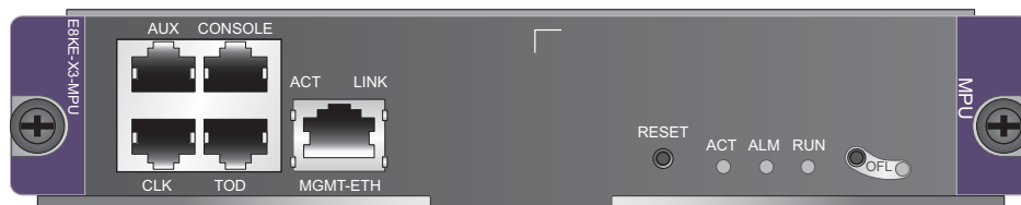
Figure 1-57 Appearance of the E8KE-X3-MPU
